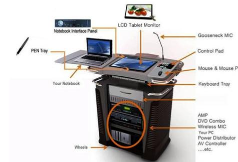
2x2 VGA switcher, audio and USB switchers, 3x 2 Video switcher, 2x microphone in, 2 RS232 COM ports. LAN hub, 1 power socket switch, 2 up/down switches for projection screen, lift, 4 auxiliary relay switches, 3 IR control outputs.
