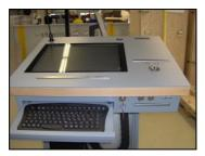
The touch screen has been inserted surface-flush in the vertical column.
