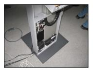
The base plate enables flexible use of the terminal at different locations. It is firmly screwed to the base column. On the underside there are three apertures to lead cables out or directly into a floor tank.
