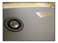
Normally microphone preparation left and right of the display includes two antivibration fixtures of Sennheiser to reduce shock transfers to the microphone. On request, one fixture integrated centrally is possible.
