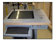
The multimedia upgrade includes a surface-flush integrated LCD flat screen in 17 inch format. In standard design this is protected from vandalism by coated protective glass.
