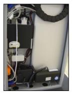
The optional PC is located on the left half of the base column. It is fastened to the base of the console vertically via a special fixture.
