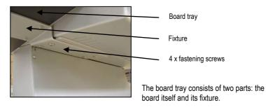
When not in use, and for transport, the board tray can be stored in the base column. On the inside of the service doors there are 4 metal bolts to fasten it.
