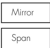
This group of keys sets up the external display or projector. Mirror will show the same image as on the system display, Span will extend the system desktop to the connected projector or external display. In the current version, these keys are NOT defined. The Display out header key will bring up the embedded graphics controller interface, so that extended desktop or mirror can be set up manually.
