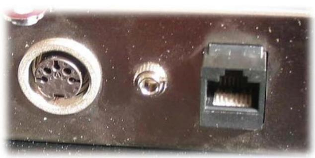
The RPT3 RJ45 has 4 circuits on its 8 connectors that are opened or closed by the relays for any need.
