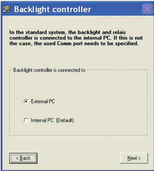
When the ILS22 is delivered in a standard setup, an internal PC is used to control the system and the backlight and relays controller. The internal PC has 4 serial comm ports, of which COM4 is used to communicate with the backlight controller (see above scheme). In situations where an external PC is used, ILStranlator needs to know to which serial port will be used to address the backlight controller inside the ILS22.
