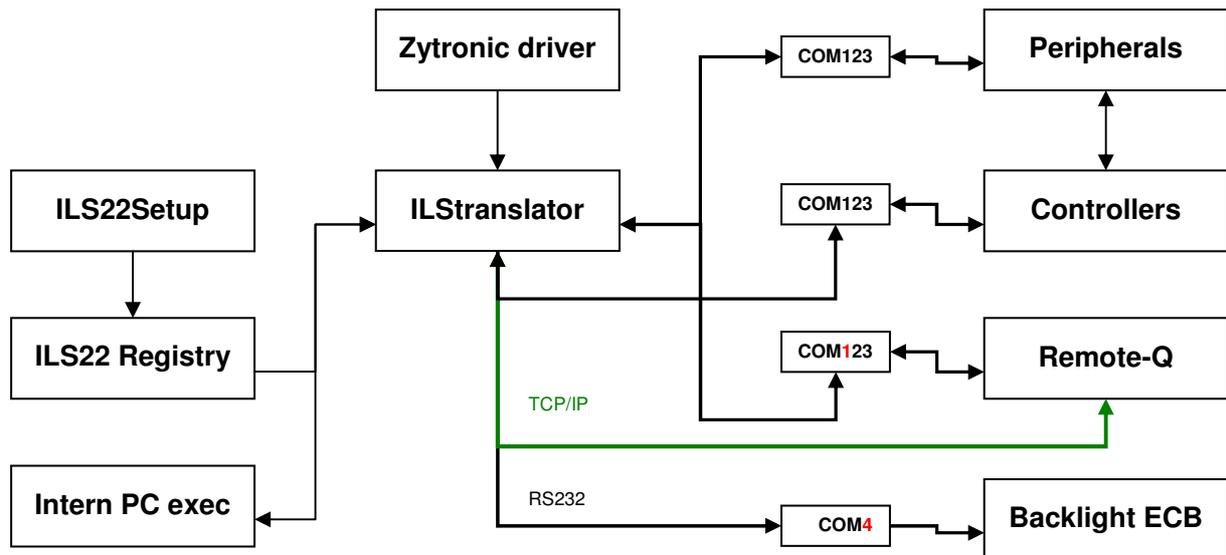
Via Com1, Com2 or Com3, ILStranlator can directly control projectors or other peripherals, or pass control over to intelligent attached controllers, which in turn can control the environment. Use the ILS22Setup Wizard to define the system setup.
