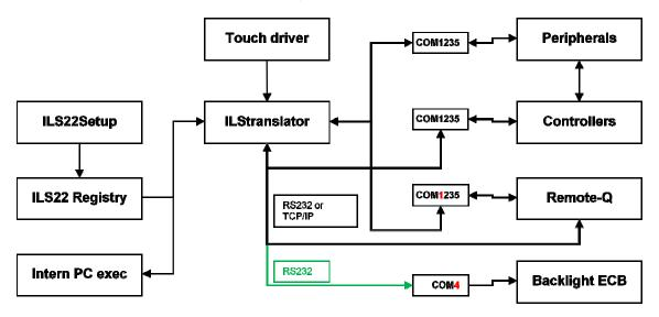
Via Com1, Com2, Com3 or Com5, ILStranslator can directly control projectors or other peripherals over a RS232 connection, or pass control over to intelligent attached controllers, which in turn can control the environment. Use the ILS22Setup Wizard to define the system setup.
