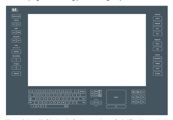
Where as the inner-side of the glass-plate functions as touch-screen for the LCD and the operating system, the outer sides (left, bottom and top) contain engraved headers and buttons for additional functions and the integrated keyboard. These functions are available to the presenter if they are visible with the backlight turned on.
